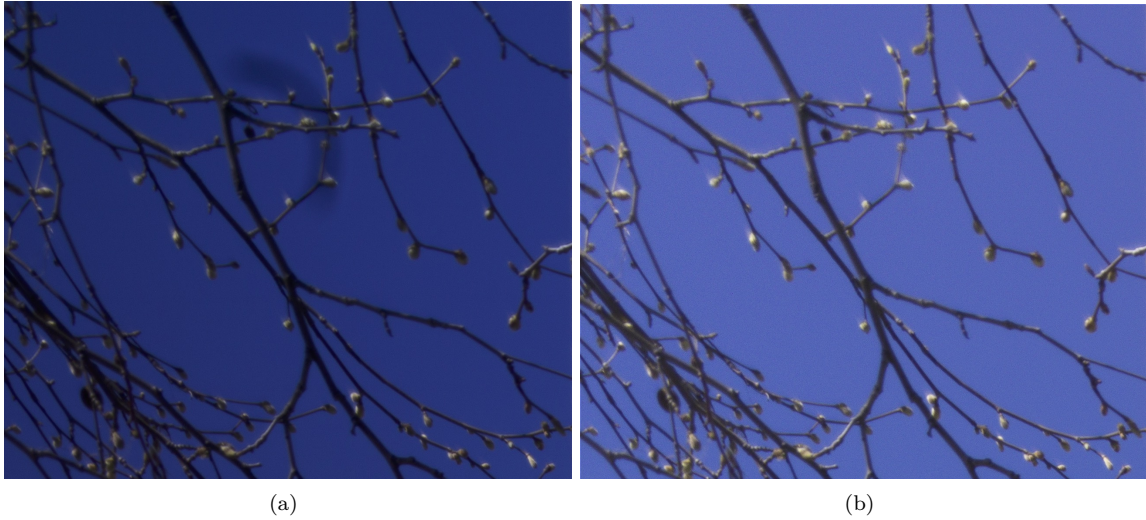
Figure 11: (a) Original image - dust spot and vignetting present (b) Processed image - dust spot and vignetting corrected
