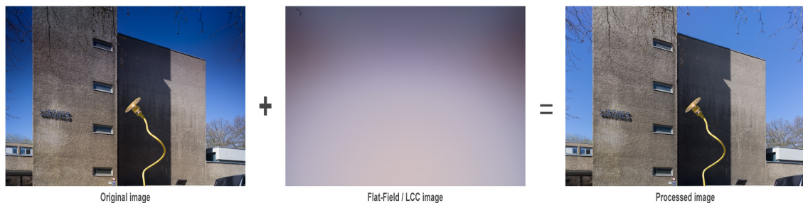
Figure 9: Flat-field application process
