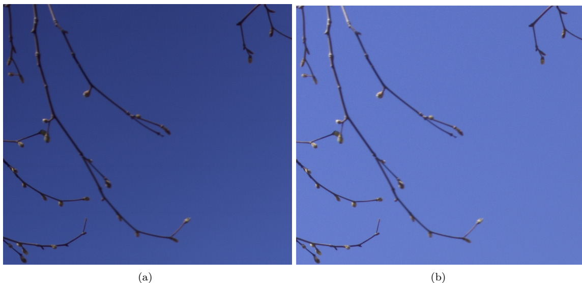
Figure 10: (a) Original image - horizontal PDAF banding and vignetting present (b) Processed image - horizontal PDAF banding and vignetting corrected
