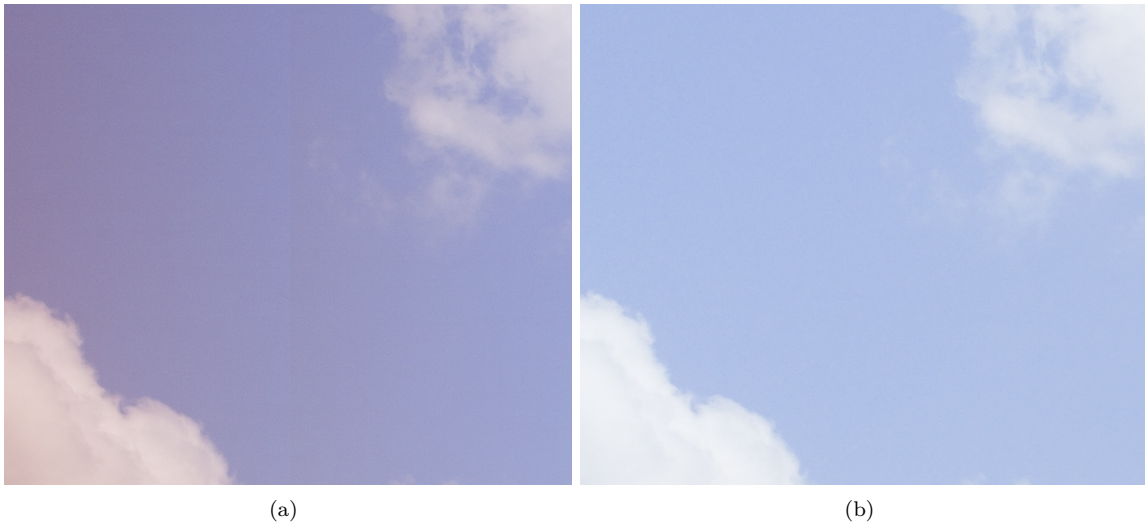
Figure 12: (a) Original image - sensor tiling, color cast and vignetting present (b) Processed image - sensor tiling, color cast and vignetting corrected
