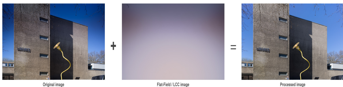
Figure 10: Flat-field application process
