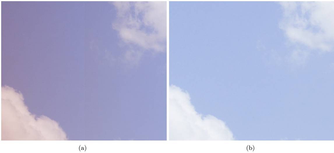
Figure 13: (a) Original image - sensor tiling, color cast and vignetting present (b) Processed image - sensor tiling, color cast and vignetting corrected
