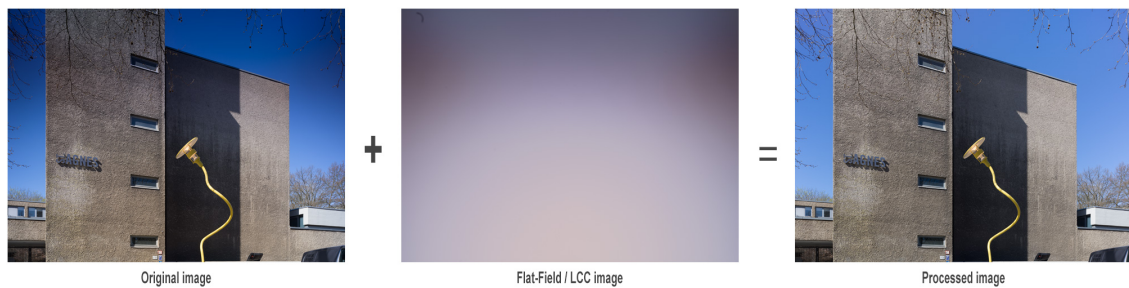
Figure 11: Flat-field application process
