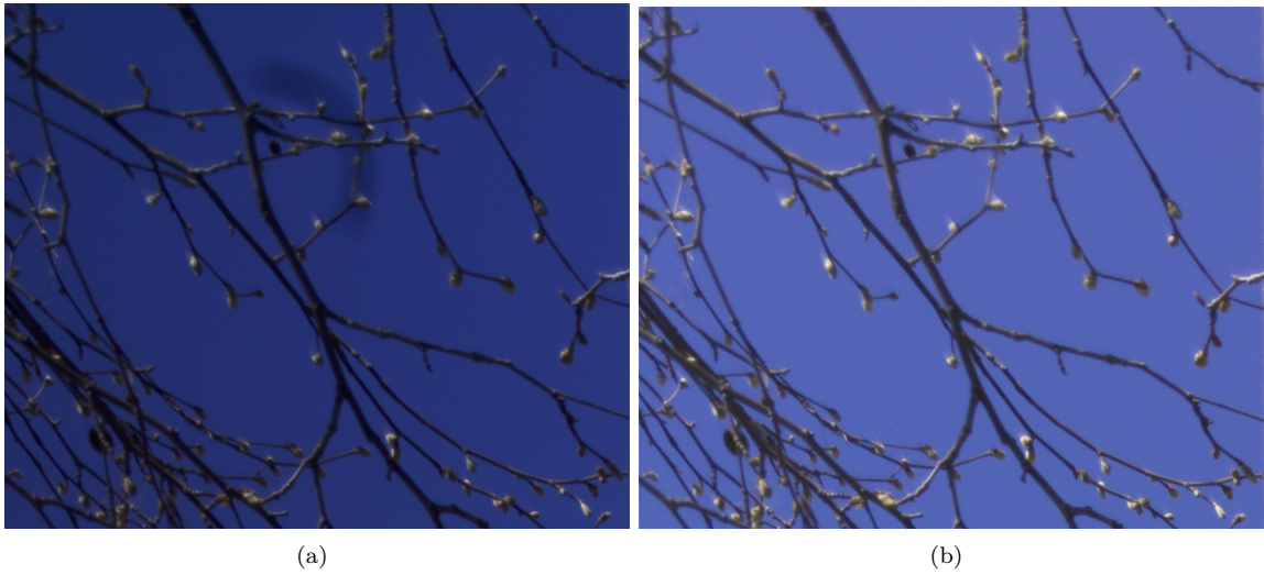
Figure 16: (a) Original image - dust spot and light falloff present (b) Processed image - dust spot and light falloff corrected
